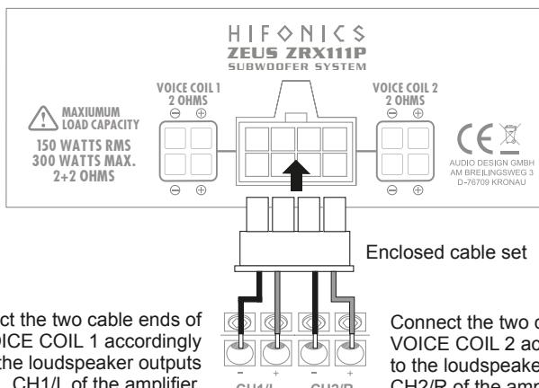
Connect the two cable ends of
